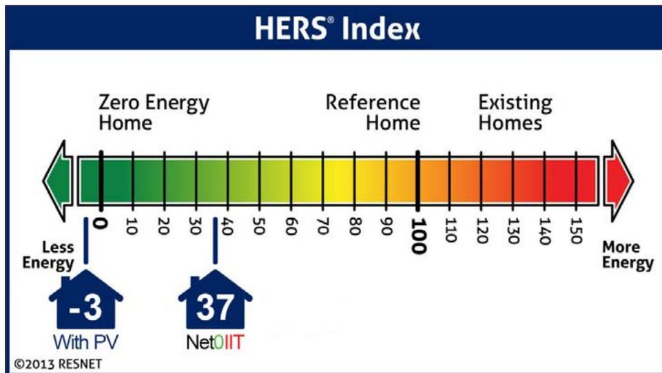
Home Energy Rating System(HERS) Index is the industry standard for measuring energy efficiency of a home. It was calculated using the software REM/Rate. A rating of 100 is the standard for new homes. We were able to get a HERS score of 37 without PV. It signifies that our home was 63% more efficient than a standard new home of the same shape and size. With the installation of PV systems, the HERS score lowered down to -3.
