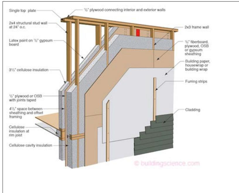
Figure 1. Example double stud wall enclosure detail from Building Science Corporation. Note that the 1/2" OSB sheathing between the two double stud cavity layers is replaced by 3.5" of rigid XPS insulation in our detail.
